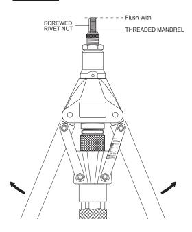
**NOTE:** After adjusting the Protruding Length (L) of THREADED MANDREL, the Screwed RIVET NUT should be flush with the Top of THREADED MANDREL.
