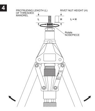
As the Stroke Distance has been re-adjusted, the Protruding Length (L) of THREADED MANDREL needs to be adjusted again to be same as RIVET NUT Height (H), L = H, as per the above "G" instruction.
