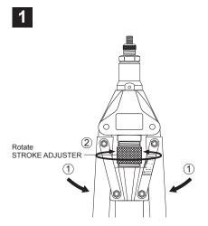
Close 2 HANDLES completely ①, rotate STROKE ADJUSTER ② to adjust the proper Stroke Distance in 2 popular ways.
