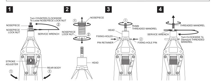
Close 2 HANDLES completely by turning down STROKE ADJUSTER until it touches the REAR BODY 1. Use SERVICE WRENCH to loose NOSEPIECE LOCK NUT by turning Counter-Clockwise 2.
