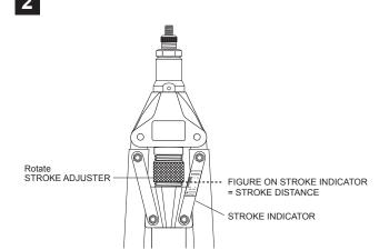
First Way: Rotate STROKE ADJUSTER to find out the Figure on the STROKE INDICATOR parallel with the Bottom Edge of the STROKE ADJUSTER:
