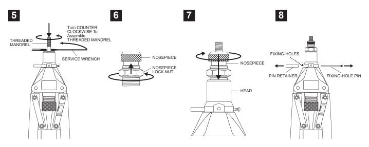
Use Hand and SERVICE WRENCH to assemble the working size of THREADED MANDREL into MANDREL SEAT firmly by turning Counter-Clockwise. ( NOTE: MANDREL SEAT has
