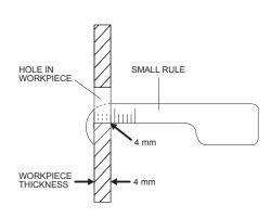
**NOTE:** The SMALL RULE is specially designed to measure the WORKPIECE Thickness.
