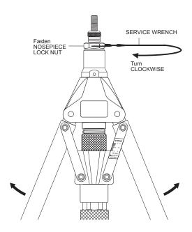
Finally use SERVICE WRENCH to fasten NOSEPIECE LOCK NUT by turning Clockwise.
