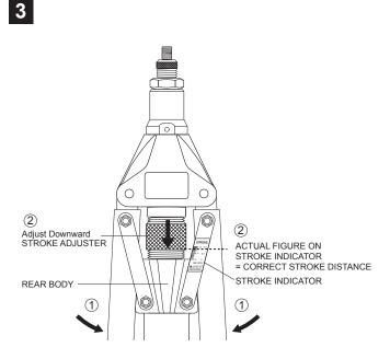
Close 2 HANDLES completely ① to touch REAR BODY, and adjust the STROKE ADJUSTER downward to let Bottom Edge of STROKE ADJUSTER parallel with the "Actual Figure on STROKE INDICATOR" ②. Now the correct Stroke Distance has been re-adjusted.
