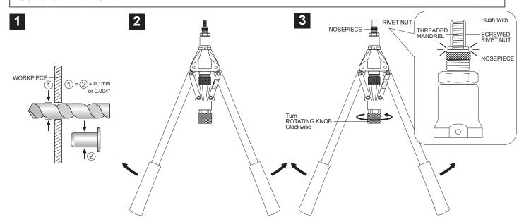
Drill or punch a Hole on WORKPIECE, Hole diameter (1) should be 0.1 mm or 0.004" larger than RIVET NUT diameter (2).
