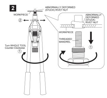
Turn whole TOOL Counter-Clockwise to unscrew THREADED MANDREL from the Stuck RIVET NUT①. Finally, take off PIN RETAINER and pull FIXING-HOLE PIN from the FIXING-HOLES②.
