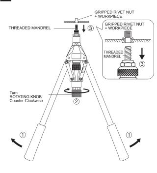
Open 2 HANDLES fully ①, turn ROTATING KNOB Counter-Clockwise ② to unscrew THREADED MANDREL from the Gripped RIVET NUT completely ③.
