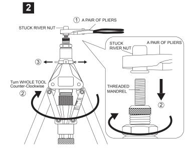
One person uses A Pair of Pliers to clamp the Stuck RIVET NUT ①, and another person turns whole TOOL Counter-Clockwise to unscrew the THREADED MANDREL from the Stuck RIVET NUT ②. Finally, take off PIN RETAINER and pull FIXING-HOLE PIN from the FIXING-HOLES ③.
