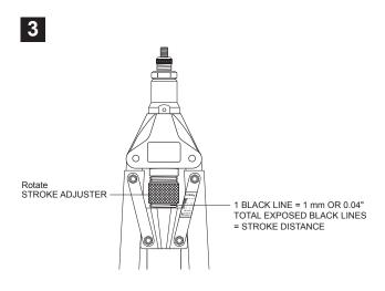
Second Way: Rotate STROKE ADJUSTER to find out the Total Exposed Black Lines of the STROKE INDICATING LINES:
