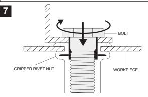
Complete the fastening work with a Bolt or a Screw to the Gripped RIVET NUT.
