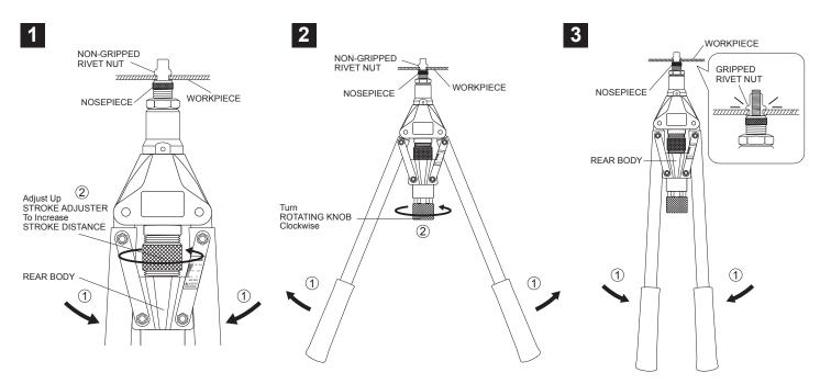
Still hold to squeeze 2 HANDLES to touch REAR BODY ①, adjust the STROKE ADJUSTER upwards ② to increase the Stroke Distance 1.0mm or 0.04" step by step.
