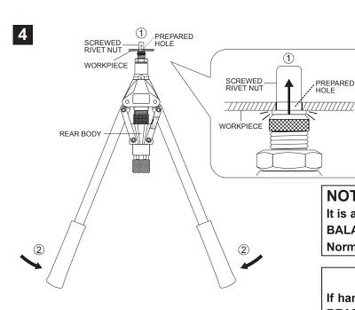
Insert the Screwed RIVET NUT into the Prepared Hole of WORKPIECE to touch WORKPIECE 1. Squeeze 2 HANDLES to touch REAR BODY 2), that drives THREADED MANDREL downwards (3) to deform RIVET NUT a Bulge against the back of WORKPIECE to fasten RIVET NUT in the WORKPIECE.
