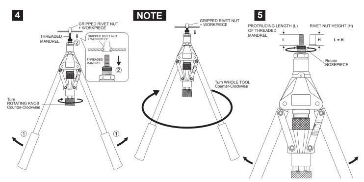
Open 2 HANDLES fully ①, turn ROTATING KNOB Counter-Clockwise to unscrew THREADED MANDREL from the Gripped RIVET NUT and WORKPIECE ②.
