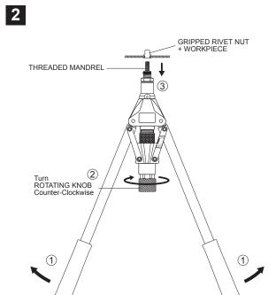
Open 2 HANDLES fully ①, turn ROTATING KNOB Counter-Clockwise ② to unscrew THREADED MANDREL from the Gripped RIVET NUT and WORKPIECE ③.
