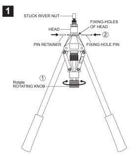
Rotate ROTATING KNOB to align the FIXING-HOLES of HEAD with the inside LONG FIXING-HOLE of MANDREL SEAT ①, then plug the FIXING-HOLE PIN into these FIXING-HOLES and put the PIN RETAINER onto FIXING-HOLE PIN End ②, the free rotation of THREADED MANDREL is therefore stopped.
