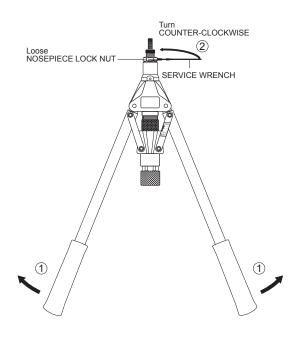
Open 2 HANDLES fully ①, use SERVICE WRENCH to loosen NOSEPIECE LOCK NUT by turning Counter-Clockwise ②.
