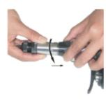
2. Turn the locknut anti-clockwise and turn the outer sleeve clockwise to shorten the stroke. Then tighten the locknut.
