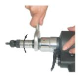
When a smaller size rivet nut is used such as M3 or M4, the stroke must be adjusted to prevent damaging the mandrel and inside thread of rivet nut.
